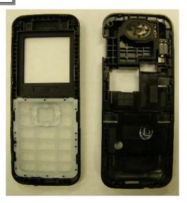
1) Assembly SPEAKER and MOTOR into the REAR.
