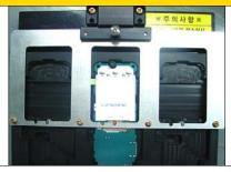
Be careful not to make Flux on the Main Board (Use the cover of Soldering Jig)
